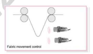
In the operation of capacitive sensors, factors such as air humidity, dust, and others can affect the switching distance. The switching distance depends on the type of target material, and the most important correction factors for different materials are shown in the table below.
