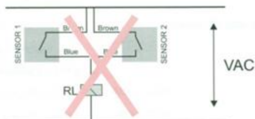
2 Wire AC sensor (not allowed)
