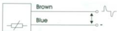
Speed pickup sensor without internal amplifier
