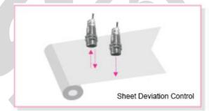
Used to monitor and control the alignment or deviation of sheets during processing by detecting shifts in the reflected infrared waves.
