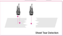
Used to identify tears or breaks in sheets (such as paper, metal, or fabric) by detecting changes in the reflected infrared waves.
