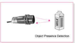
Used to detect the presence or absence of objects by sensing the reflection of infrared waves from the object's surface.
